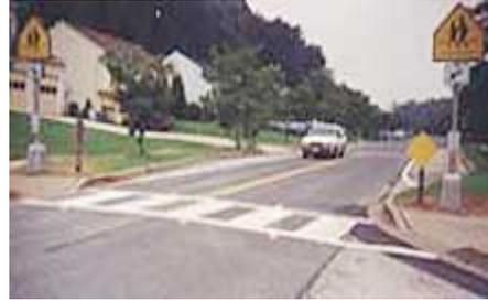
*A push button at either end of the crosswalk activates six high intensity yellow lights that flash once per second for 30 seconds. The staggered placement of TS230 fixtures maximizes visibility.*
